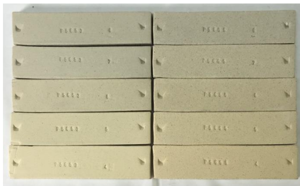
Modern clay shrinkage bars
